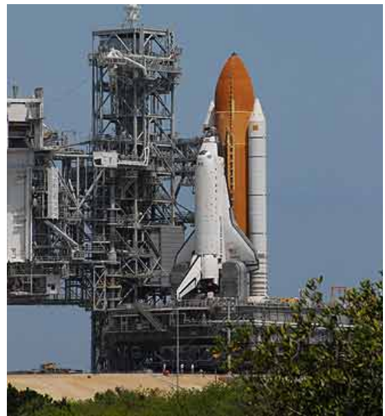
Space Shuttle Atlantis, mounted on a mobile launch platform atop a crawler transporter, sits on Launch Pad 39A awaiting flight on mission STS-117. Photo credit: NASA/Ken Thornsley.
